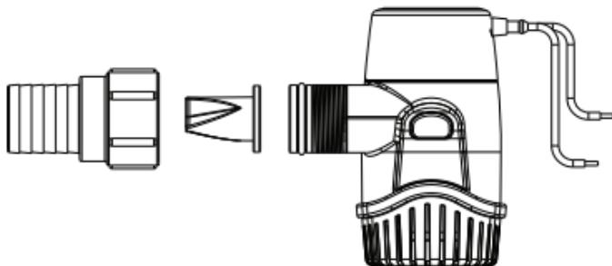
Periodically remove, clean and inspect bilge pump, check valve and its surroundings for damage or debris that may reduce the performance of the pump.
