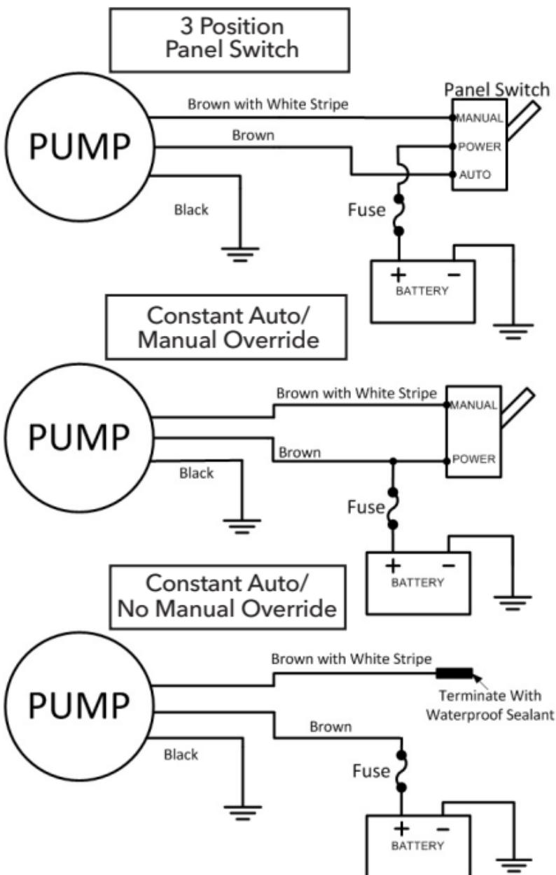
**On 12 volt pump:** Minimum voltage of 10.5 volts required.
